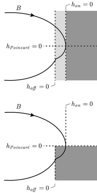
**Fig. 4** The solid trajectory in Fig. 3 is a solution to the original hybrid dynamical system with hysteresis shown in the upper panel as well as the alternative piecewise smooth dynamical system without hysteresis shown in the lower panel
