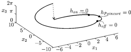
**Fig. 2** A sample periodic trajectory of the example oscillator with  $F_d \approx 6.93$ . Here, dots refer to zero-crossings of the event functions corresponding to the onset and cessation of interactions with the additional linear spring and the Poincaré sampling trigger function. The dashed line refers to the instantaneous change in  $x_3$  from  $2\pi$  to 0 that results from its definition.
