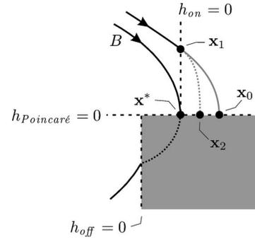
**Fig. 5** The discontinuity-mapping  $\mathbf{D}: \mathbf{x}_0 \mapsto \mathbf{x}_2$  accounts for the correction to the local flow. Here, solid curves correspond to the  $\Phi_{\text{off}}$  flow and dashed curves correspond to the  $\Phi_{\text{on}}$  flow.
