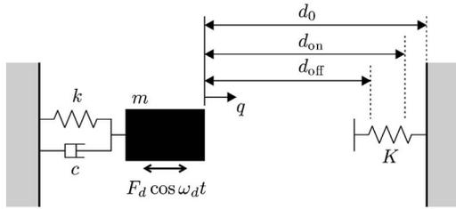
**Fig. 1** A schematic of an example oscillator. Two distinct regimes of interaction between the mass and its environment are represented by the additional spring with stiffness  $K$  and zero load when  $q=d_0$ . Here,  $d_{on}$  denotes the displacement of the mass at which the spring is initially engaged and  $d_{off}$  denotes the displacement of the mass at which the spring is disengaged.
