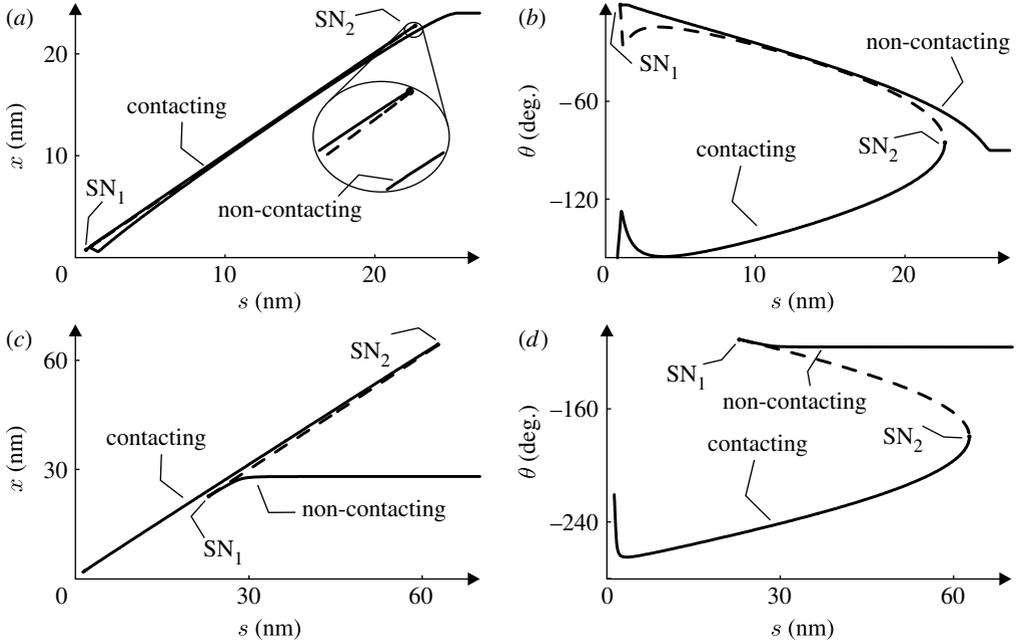
Figure 1. Changes in the maximum deviation between the cantilever tip and the sample surface and in the corresponding phase lag under changes in the equilibrium separation distance for (a,b) the piecewise-linear and (c,d) the piecewise-nonlinear force models. Dashed lines indicate unstable oscillations, while solid lines indicate stable oscillations. The corresponding branches of periodic solutions are connected through two saddle-node bifurcation points at  $SN_1$  and  $SN_2$ .
