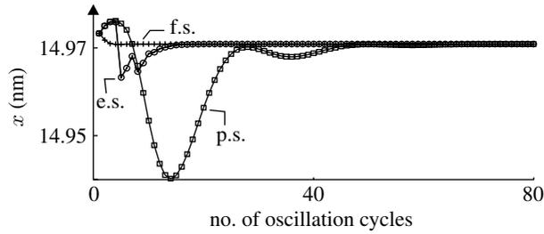
Figure 4. Comparison between the convergence properties of the full-state (f.s.), estimated-state (e.s.) and partial-state (p.s.) feedback approaches near an unstable periodic oscillation in the piecewise-linear tip-sample interaction model.
