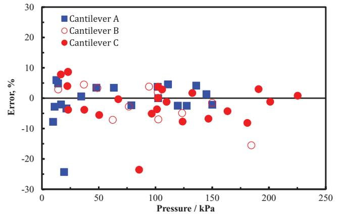
FIG. 3. Percentage error of cantilever-gauge pressure from the commercial-gauge pressure in the range 10–225 kPa. The error is calculated as  $1 - (\text{cantilever-gauge pressure}/\text{commercial-gauge pressure})$ . Except for three data points, the errors are within 10%. The mean error is 5%.
