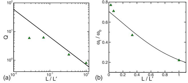
FIG. 7. (Color online) The variation in the quality  $Q$ , panel (a), and of the resonant frequency in fluid  $\omega_f/\omega_0$ , panel (b), by decreasing the length  $L$  of the beam relative to the value of case (1) given by  $L'$ . The triangles are the results from numerical simulation and the solid line is the analytical prediction.
