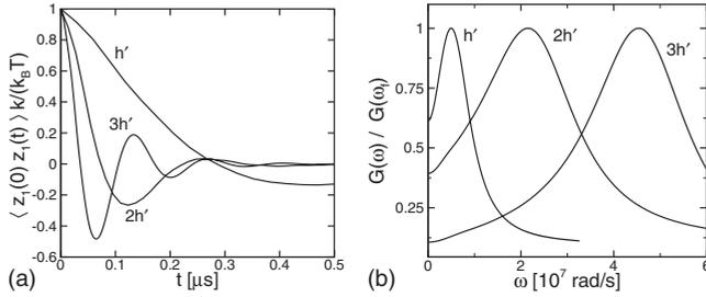
FIG. 5. The autocorrelations and noise spectra as a function of beam height from numerical results: case 1 ( $h'$ ), case 4 ( $2h'$ ), case 5 ( $3h'$ ). (a) The normalized autocorrelations. (b) The normalized noise spectra.
