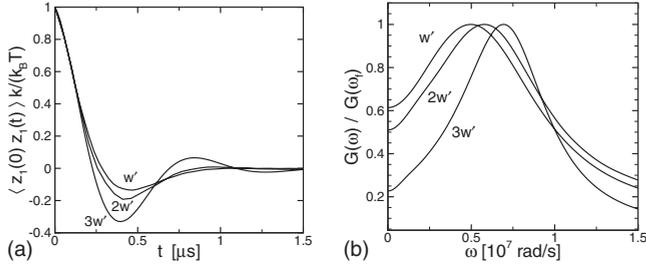
FIG. 3. The autocorrelations and noise spectra of equilibrium fluctuations in beam displacement as a function of beam width from numerical results: case 1 ( $w'$ ), case 2 ( $2w'$ ), case 3 ( $3w'$ ). (a) The autocorrelations, the results have been normalized using  $k/(k_B T)$  for each case. (b) The noise spectra, the results have been normalized by the peak value for each case,  $G(\omega_f)$ .
