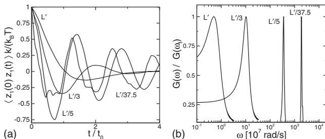
FIG. 6. The autocorrelations and noise spectra as a function of beam length from numerical results: case 1 ( $L'$ ), case 6 ( $L'/3$ ), case 7 ( $L'/5$ ), case 8 ( $L'/37.5$ ). (a) The normalized autocorrelations. (b) The normalized noise spectra.
