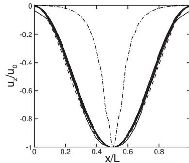
FIG. 8. The transverse fluid velocity  $u_z$  for cases 1–8 along the line beginning at  $(0,0,0,0.01 \mu\text{m})$  and ending at  $(L,0,0,0.01 \mu\text{m})$  from the deterministic numerical simulations where the beam velocity is at its maximum value. The baseline geometry is shown as the dashed line, cases 2–7 are the solid lines, and case 8 is the dash-dot line.
