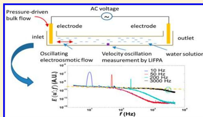
In micro- and nanofluidic systems, due to the large surface-to-volume ratio, electroosmotic flow (EOF) has been widely used to pump fluids and manipulate objects for various applications, such as DNA transport, hybridization and separation in biomedical engineering, and enhancing heat and mass transfer.<sup>1–5</sup>
