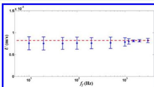
**Figure 6.** Mean velocity of flow under different forcing frequencies measured at a near wall position of  $z = 2 \mu\text{m}$ . The flow rate is  $Q = 2 \mu\text{L}/\text{min}$ .  $E_A = 2 \times 10^3 \text{ V}/\text{m}$ . The red dashed line indicates the mean velocity ( $\approx 0.8 \text{ mm}/\text{s}$ ) of the unforced flow.
