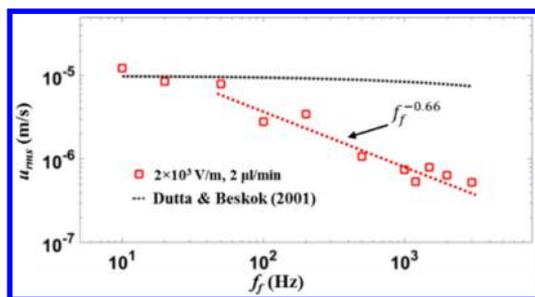
**Figure 8.**  $u_{\text{rms}}$  varies with  $f_f$ . The experimental data (red square) at  $z = 2 \mu\text{m}$  is compared with theoretical prediction (black dotted line) by Dutta and Beskok.<sup>20</sup> Note, the influence of the low-pass filter has been corrected as introduced in the main text.
