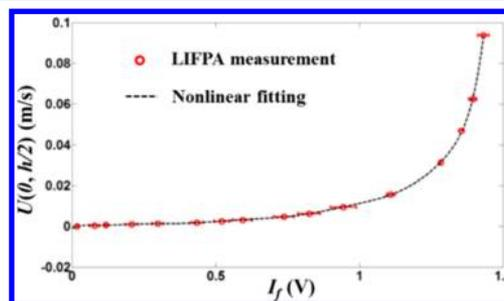
**Figure 4.** Typical velocity calibration curve measured at the center of microchannel. The velocity is calculated from the flow rate by eq 2. The calibration curve is nonlinearly fitted by polynomial series.
