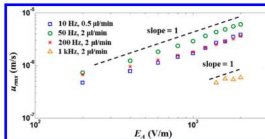
**Figure 9.**  $u_{\text{rms}}$  varies with applied electric field intensity at different  $f_f$  and  $Q$  at  $z = 2 \mu\text{m}$ . The dashed lines show the slope of power law curve. Note, the influence of low-pass filter has been corrected as discussed in the third section of the Discussion.
