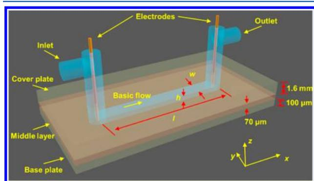
**Figure 1.** Schematic of the microchannel.  $x$ ,  $y$ , and  $z$  represents streamwise, spanwise, and vertical directions, respectively.
