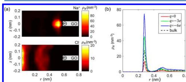
**Figure 7.** (a) Distribution of  $\text{Na}^+$  ions (upper panel) and  $\text{Cl}^-$  ions (lower panel) inside and near a large pore with  $q = -6e$ .  $z = 0$  and  $r = 0$  denote the pore's horizontal plane and vertical axis, respectively. (b) Radial density distribution of  $\text{Cl}^-$  ions around the  $\text{Na}^+$  ions inside the large pore with different charge  $q$  and in bulk 2 M NaCl solution.
