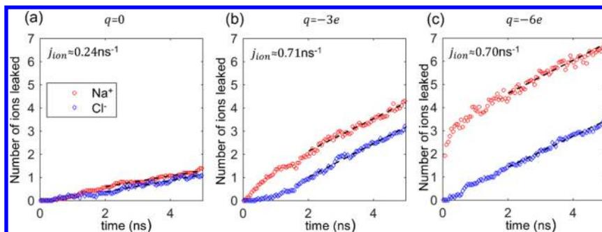
**Figure 6.** Evolution of the number of ions leaked through large pores (nominal diameter: 1.12 nm) with net charge  $q = 0, -3e$ , and  $-6e$ . The dashed lines denote linear regression at time larger than 2 ns. A pressure difference of 50 MPa between the salt and fresh water sides is used to drive the water transport.
