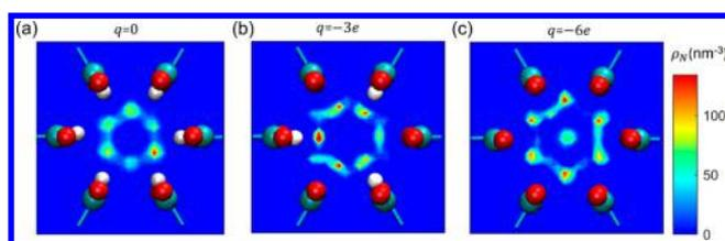
**Figure 3.** The  $xy$ -plane distribution of water molecules inside the small pore with a nominal diameter of 0.68 nm. The pore's net charge is  $q = 0$ ,  $-3e$ , and  $-6e$  in the three panels. The carboxyl groups (neutral and ionized) along the pore's perimeter are shown as van der Waals spheres (hydrogen, oxygen, and carbon atoms are in white, red, and cyan color, respectively).
