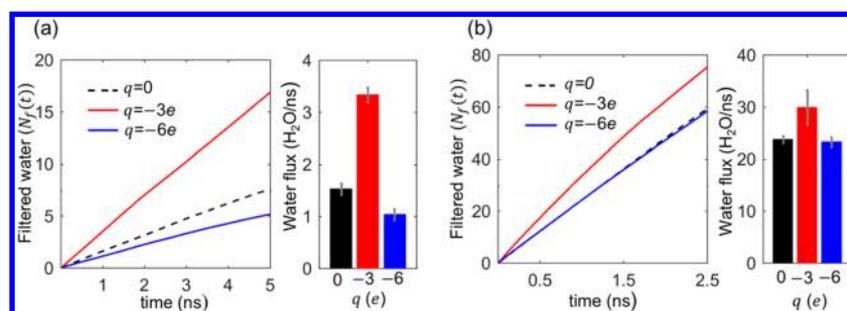
**Figure 2.** The accumulative number of water molecules filtered through nanopores with different size and charge and the corresponding water flux. (a) Small nanopores with a nominal diameter of 0.68 nm. (b) Large nanopore with a nominal diameter of 1.12 nm. A pressure difference of 100 and 50 MPa between the salt and fresh water is used to drive the water transport through the small and large nanopore, respectively.
