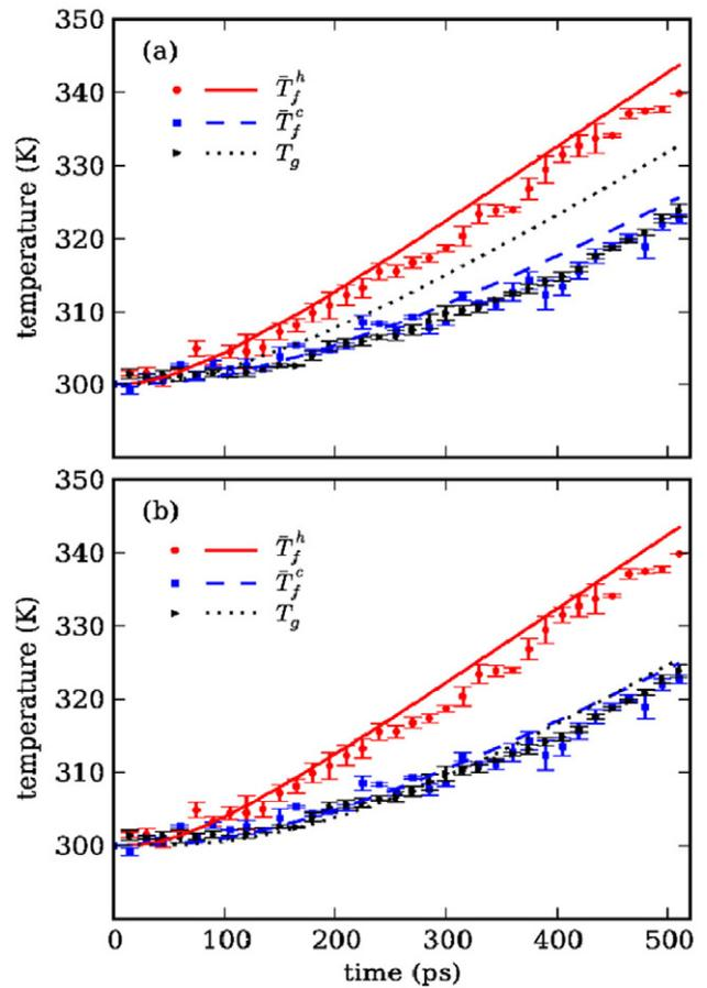
**Figure 2.** Evolution of the temperature of the graphene sheet and the octane fluids in the observation windows shown in figure 1(a) during the transient heating simulations described in the text. The predictions of the MD simulations (filled symbols) are compared with those by the continuum simulations (thin lines) based on the Kapitza model (a) and on the nonlocal model (b).
