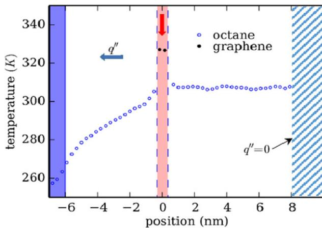
**Figure 3.** Temperature profiles of the octane fluids and the graphene sheet shown in figure 1. Heat is injected into the graphene sheet and removed from the octane fluids in the purple shaded region ( $-7 \text{ nm} < x < -6 \text{ nm}$ ). The two vertical dashed lines denote the two surfaces of the graphene sheet.
