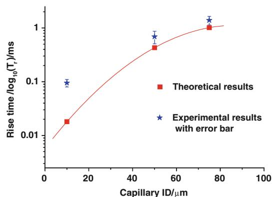
**Fig. 3** Comparison of the measured  $t_r$  on the axis in microcapillaries having ID of 10, 50, and 75  $\mu$ m, respectively, with theoretical prediction. (Note: the experimental data for 50 and 75  $\mu$ m ID are obtained from another work (Kuang et al. 2009a) in order to compare the influence of ID on the rise time  $t_r$  of EOF)
