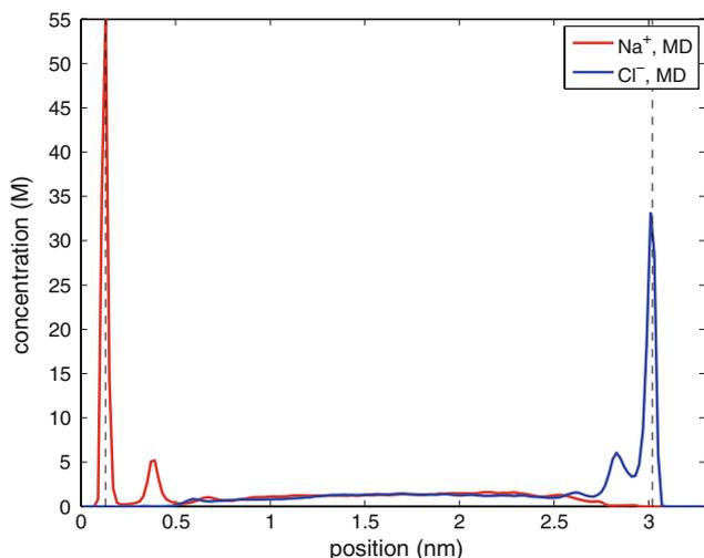
**Fig. 4** Equilibrium ion concentration between two electrodes with charge densities of  $-0.26\text{C/m}^2$  and  $0.26\text{C/m}^2$ , respectively. The bin size used for computing the ion concentration is 0.02 nm
