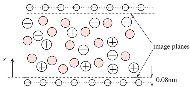
**Fig. 1** A schematic of the MD simulation system. The empty circles denote the electrode atoms and the filled circles denote water molecules
