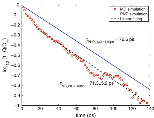
**Fig. 3** Charging kinetics for the EDLs between two electrodes computed by using MD simulations and by using the PNP/Stern model. The voltage difference between the two electrodes is 2 Volts
