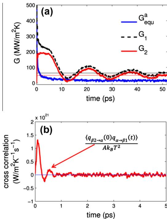
**Fig. 4 – (a) Running integration of  $G_{equ}^a$ ,  $G_1$ ,  $G_2$  given by Eqs. (7a)–(7c). (b) Cross-correlation function  $\langle q_{\beta 2 \rightarrow \alpha}(0) q_{\alpha \rightarrow \beta 1}(t) \rangle$  in Eq. (7c). The graphene sheet is a single-layer graphene. (A colour version of this figure can be viewed online.)**
