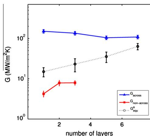
**Fig. 3 – Interfacial thermal conductance at graphene–octane interfaces probed using various methods for the systems shown in Fig. 1. (A colour version of this figure can be viewed online.)**
