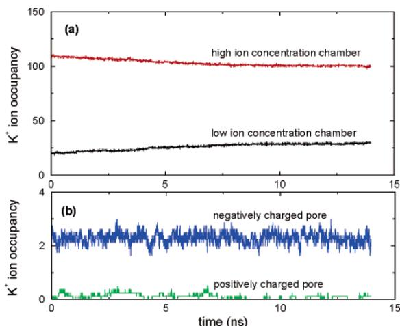
**Figure 4.** Evolution of the  $K^+$  ion occupancy in the two solution chambers (a) and in the membrane pores (b) with time.
