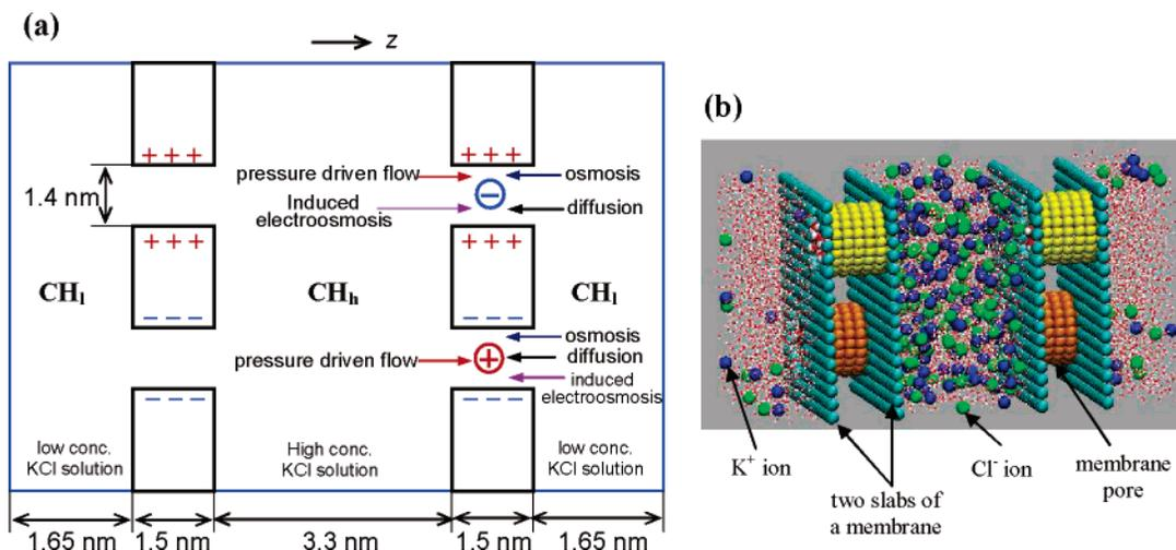
**Figure 1.** (a) Sketch of the simulation system. The various physical mechanisms, along with their directions, that could play a role in the transport of water are represented by arrows, and the water recirculation loop is also shown. The fluxes are symmetrical in the left membrane. CH<sub>l</sub> denotes the low ion concentration chamber, and CH<sub>h</sub> denotes the high ion concentration chamber. (b) A snapshot (rendered using VMD<sup>23</sup>) of the simulation system.
