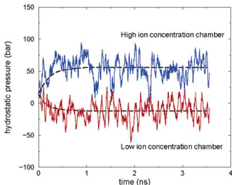
**Figure 3.** Evolution of the hydrostatic pressure in the two chambers during the first 3.5 ns of the simulation. The dashed lines are guides for the eyes.
