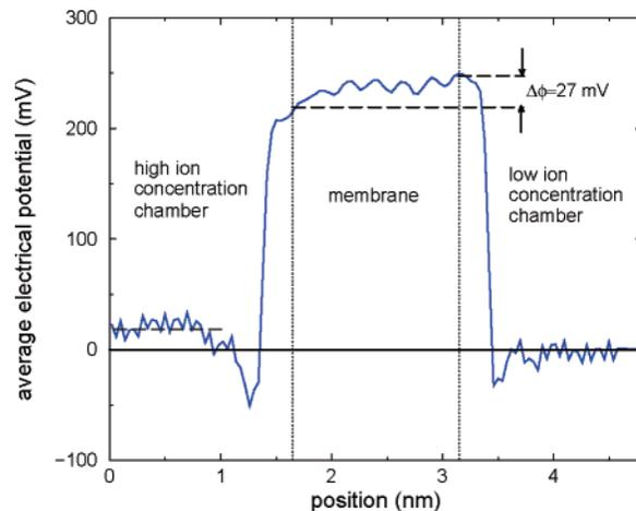
**Figure 5.** Time-averaged electrical potential ( $\bar{\phi}(z)$ ) distribution in the simulation system during 2–4 ns. Because of the symmetry of the system with respect to the plane  $z = 4.8$  nm,  $\bar{\phi}(z)$  is shown only in half of the system. The dotted lines denote the surfaces of the membrane.
