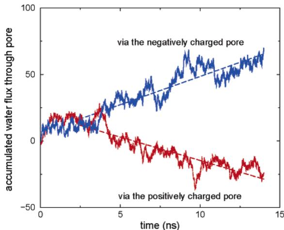
**Figure 6.** Accumulated water flux through the positive and negative membrane pores. The water flux  $\text{CH}_l \rightarrow \text{CH}_h$  (i.e., the direction of osmosis) is defined as positive. The dashed lines are a linear fit to the accumulated flux from 2 to 14 ns.
